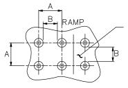
DETECTABLE WARNING PATTERN AREA SHALL BE YELLOW, AND PERPENDICULAR TO THE LONG AXIS OF THE RAMP.
