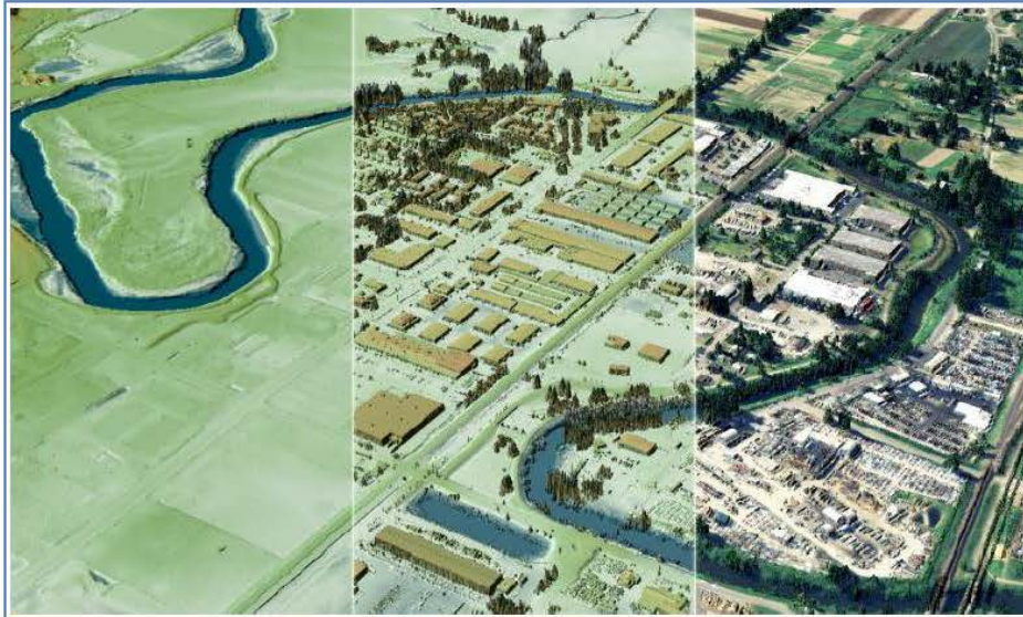
Paneled view of bare earth (L), highest hit (middle) and point cloud colored by 2013 NAIP imagery (R), Kent, WA.
